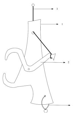
**Figure 2.** The Scheme of Fish Release Clamp (FRC) (1; main body, 2; movable clamp arm mounted on the main body, 3; steel rope, 4; lead)
