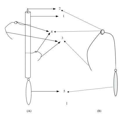
**Figure 1.** The Scheme of Fish Release Hook (FRH) (A: Use in releasing several fishes at the same time, B; Tool used in releasing a fish, 1: main body, 2: body-lashing ring, 3: needles of different size, 4: spring crimp, 5: lead)
