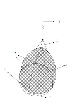
**Figure 3.** The Scheme of Fish Release Basket (FRB) (1; chrome steel frame, 2; connecting ropes, 3; part, 4; body connecting ropes, 5; main size, 6; extra weight for attaching holes)
