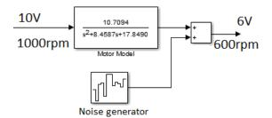
Fig. 1 The DC Motor Model with Noise
