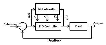
Fig. 3 Block diagram of PID optimization with ABC algorithm
