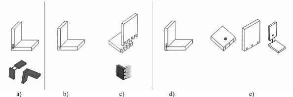
**Figure 3** Test specimens: a) Wooden dowel jointed test specimen - DJ, b) Test specimen with tongue-and-groove joint - TGJ, c) Test specimen with half-blind dovetail joint – DTJ, d) Test specimen with screw joint – SJ, and e) Test specimen with eccentric (Minifix) joint – MJ
