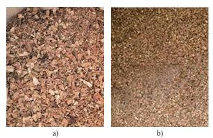
Figure 1 Peanut fibers: a) core layer fibers, b) outer layer
