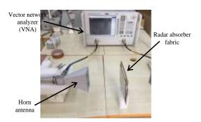
**Figure 15.** Frequency dependent reflection parameter measurements of planar radar absorber fabric
