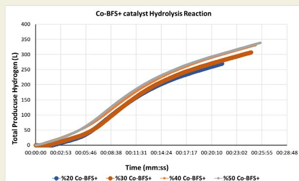
Figure 9. Hydrogen production performance graphs of Co-BFS<sup>+</sup> catalyst powders
