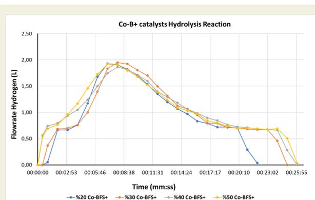
Figure 10. The flowrate hydrogen production of the Co-BFS<sup>+</sup> catalyst sample that are different amounts of Co
