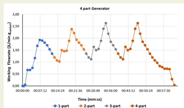
Figure 11. The performance of Autonomous Hydrogen Generator Prototype with %20 Co-BFS catalyst for 1-hour
