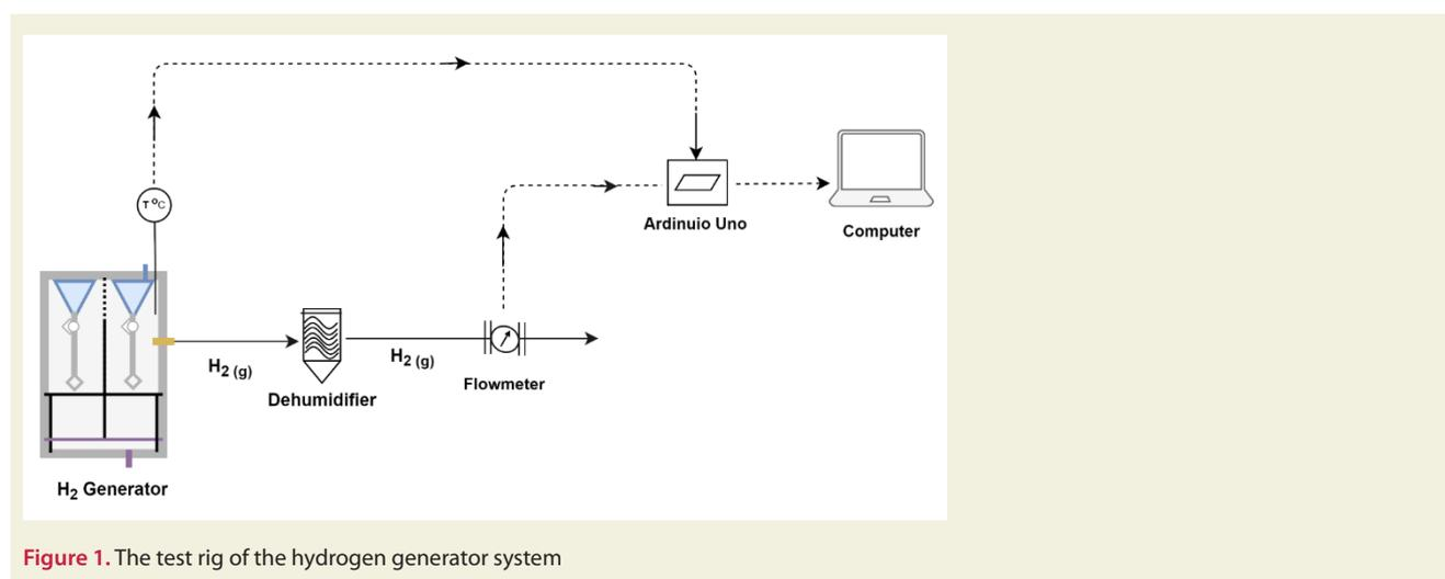
Figure 1. The test rig of the hydrogen generator system
