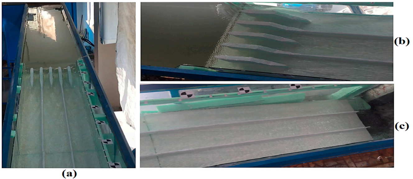
Figure 4. Model image of the spillway in the experiment: (a) top view; (b) flow inlet part; (c) flow output part.
