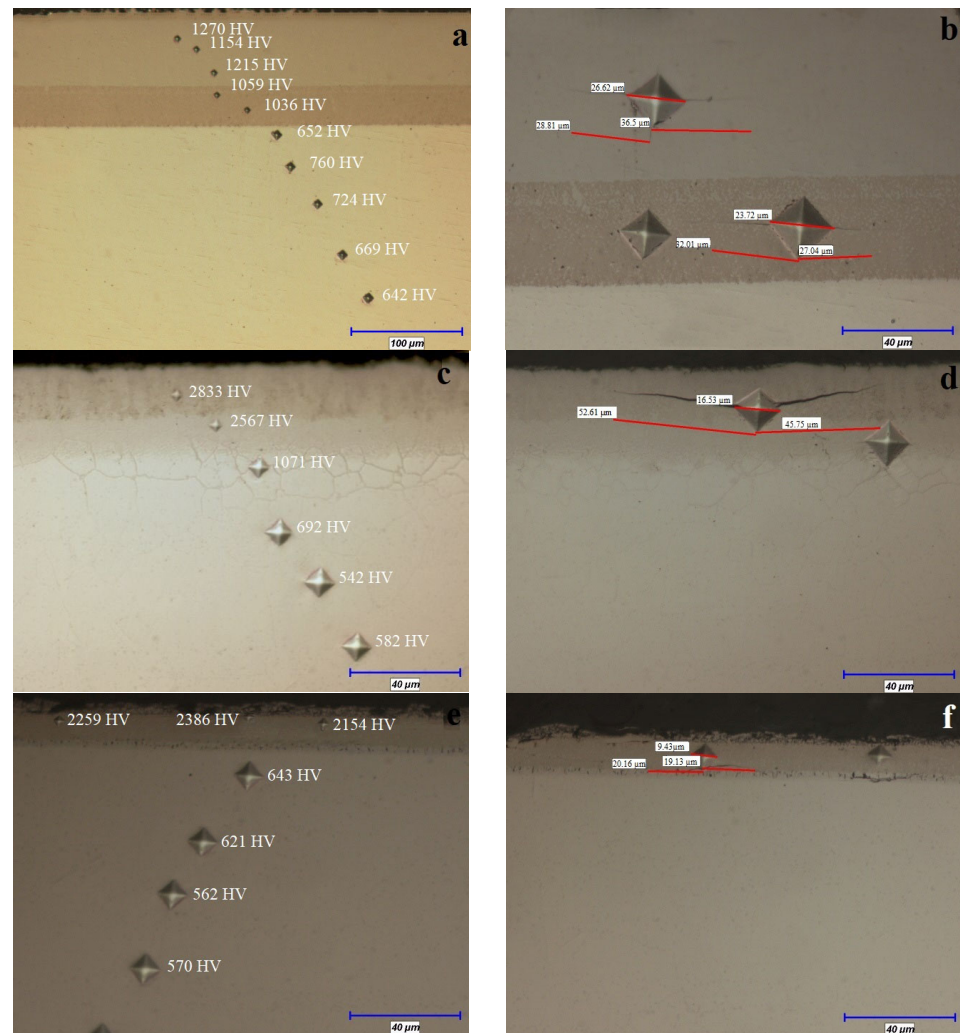
Figure 5. Hardness profiles and fracture toughness traces formed on the section surfaces. (a) Al hardness trace, (b) Al fracture toughness trace, (c) B hardness trace, (d) B fracture toughness trace, (e) Al-B hardness trace, (f) Al-B fracture toughness trace.
