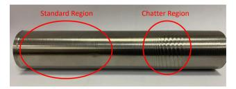
Fig. 8 Surface roughness after turning for Ti6Al4V workpiece
