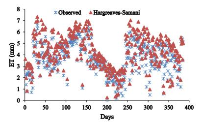
Fig. 4. Distribution graph of Hargreaves-Samani equation test results
