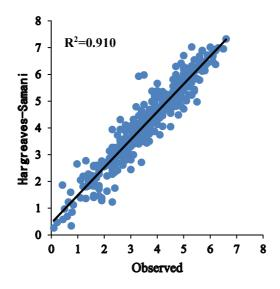
Fig. 5. Scatter chart of Hargreaves-Samani equation test set results
