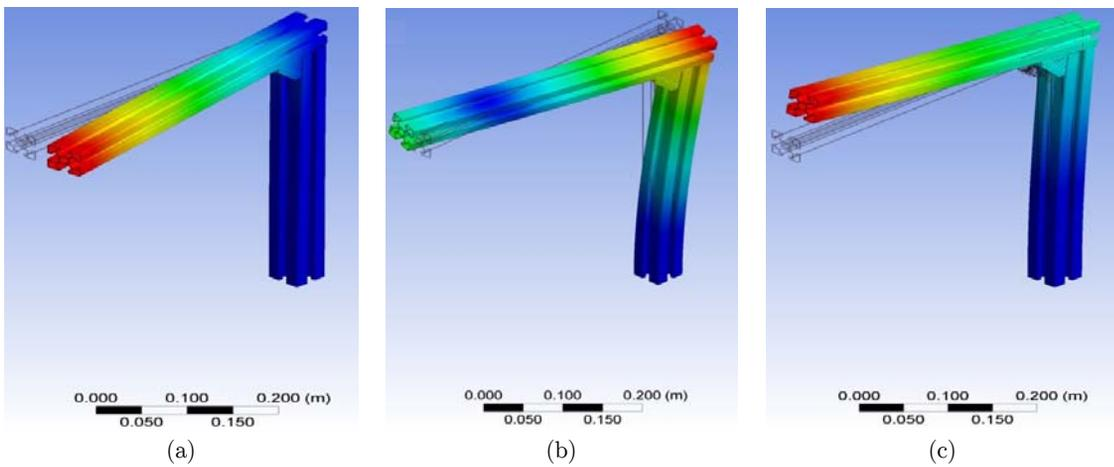
**Figure 9:** Mode shapes of LF-45 with solid finite elements for LF-45, (a) Mode-ty, (b) Mode-bx, (c) Mode-bz.
