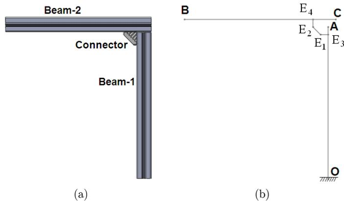
Figure 3: (a) Solid model, (b) Line model
