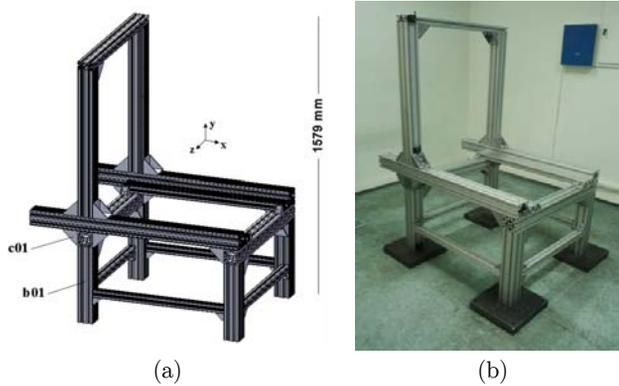
**Figure 1:** Solid model of frame of test system (a), photo of TS-1A (b).
