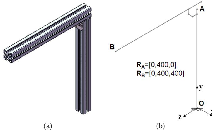
Figure 8: L-frame (LF-45) (a) Solid model for simulations (b) line model.
