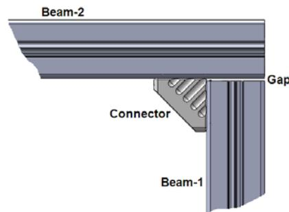
Figure 2: Gap given between connected beams
