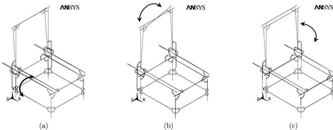
**Figure 12:** Mode shapes of Frame TS-1B, (a) Mode-bx, (b) Mode-ty, (c) Mode-bz
