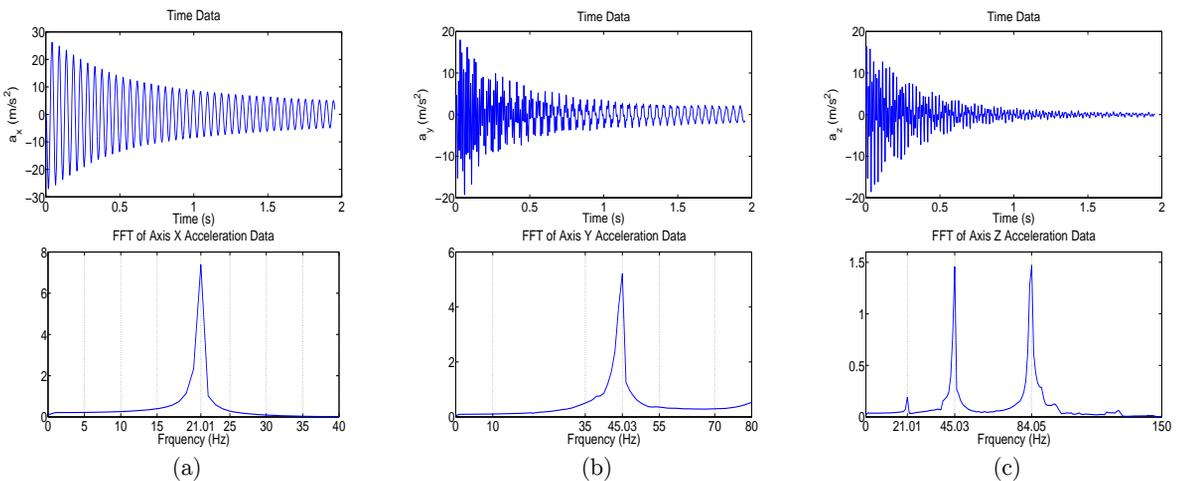
**Figure 10:** FFT's of signal components and acceleration signal for experimental results in Table 8 for (a) Mode-ty, (b) Mode-bx, (c) Mode-bz
