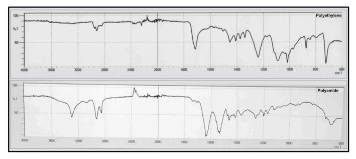
Fig. 5. Representative FTIR spectra for major identified polymers.
