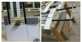
**Figure 7.** Installation of the morphing mechanism on the UAV
