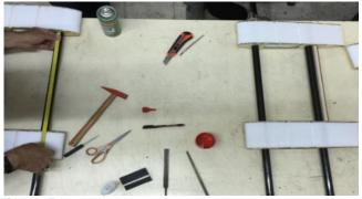
**Figure 5.** Threading the profiles of UAV into carbon pipes The measurements of the gaps on the leading edge of the wing were taken. In the light of these dimensions, a leading edge drawing was made to complete the profile. Appropriately sized styrofoams were selected. The parts drawn in the
