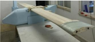
Figure 13. Wing - Body Assembly
