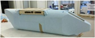
Figure 12. Covering the fuselage with foam
