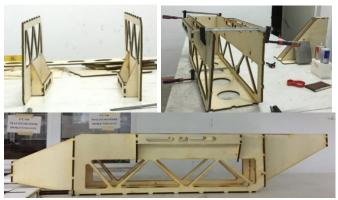
Figure 11. Fuselage Manufacturing
