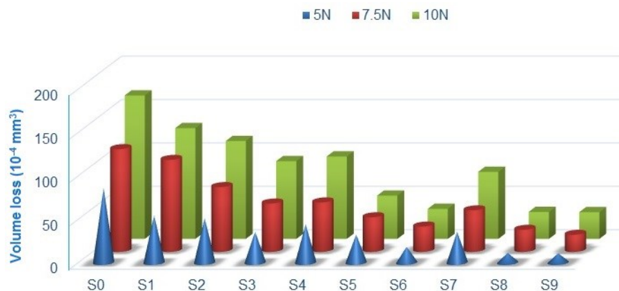
Figure 4: Volume loss of the samples subjected to fixed ball micro-abrasion wear test depending on applied load.
