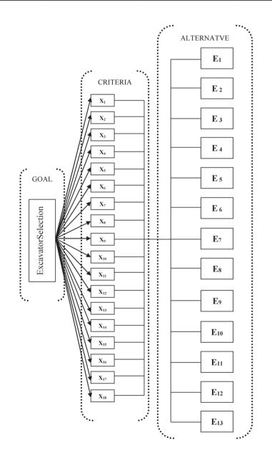
Fig. 3. Hierarchy for excavator technologies evaluation
